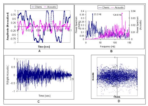
Figure 11: Time series (A), power spectrum (B),  $(R_{chemil. - acoustic})$  (C), and phase space diagram (D),  $(d_1 = 0.7mm$  and H/D=1).
