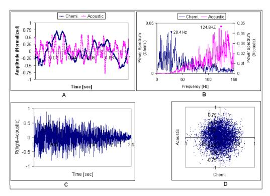
Figure 12: Time series (A), power spectrum (B),  $(R_{chemil. - acoustic})$  (C), and phase space diagram (D),  $(d_2=1.2mm$  and H/D=0.5).
