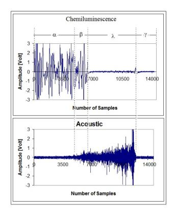
Figure 8: Time history of Chemiluminescence emission and acoustic pressure signals at H/D=1, Burner diameter 1.2mm.
