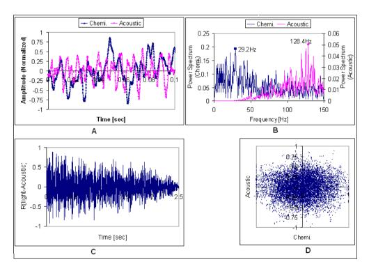
Figure 10: Time series (A), power spectrum (B), cross-correlation of ( $R_{\text{chemil.}-acoustic}$ ) (C), and phase space diagram (D)( $d_1$ =0.7mmand H/D=0.5).
