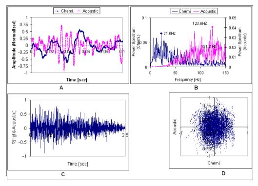
Figure 14: Time series (A), power spectrum (B),  $(R_{chemil. - acoustic})$  (C), and phase space diagram (D),  $(d_2=1.7mm$  and H/D=0.5).
