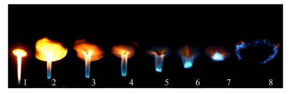
Figure 4: flame photography images during the increase of fuel flow rate from a laminar to the flame blowout conditions at H/D=1, and Burner diameter 0.7mm
