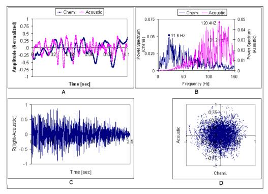
Figure 13: Time series (A), power spectrum (B),  $(R_{chemil. - acoustic})$  (C), and phase space diagram (D),  $(d_2=1.2mm$  and H/D=1).
