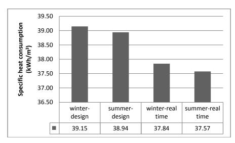
Figure 2: Specific heat consumption
