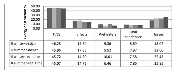
**Figure 6: Exergy destruction percentage for different operating conditions**
