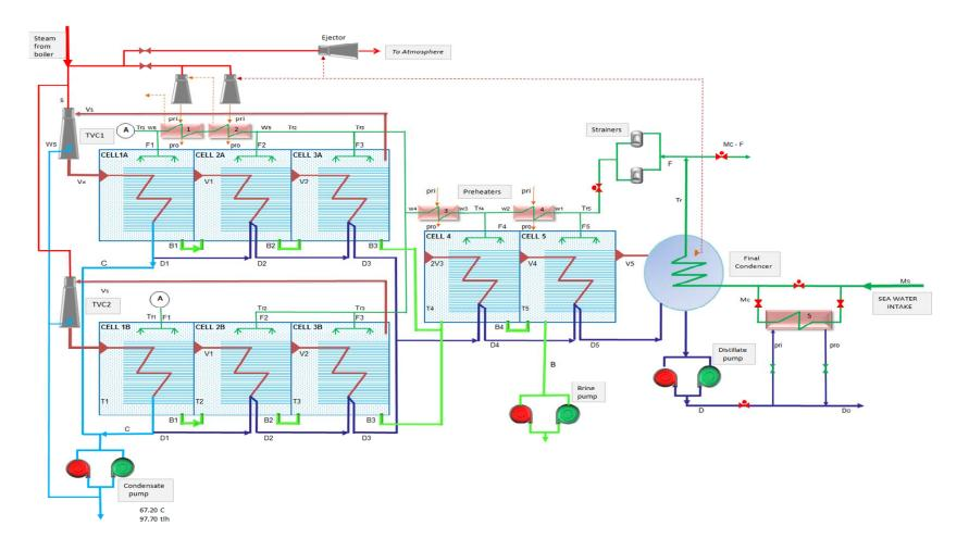
Figure 1: Schematic diagram for unit one of Zawia desalination plant
