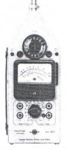
Figure 1: Impulsive Precision Sound Level Meter, B&K 2209
