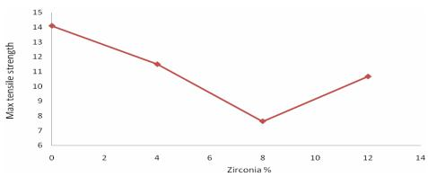
Figure 2: Effect of zirconia weight (%) on maximum tensile strength
