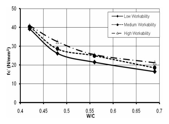
Figure 1: Test results for compressive strength of concrete samples
