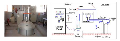
Figure 2: Gas nitriding Pit Furnace model 572 (SIB company)
