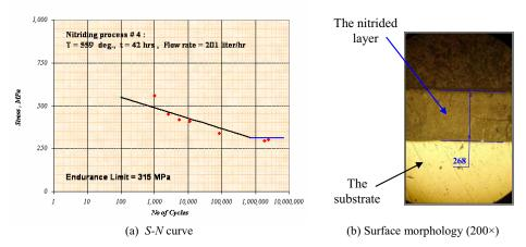
Figure 6: *S-N* curve for fatigue test and layer morphology of nitrided specimen (Design point No 4 (T = 559 °C, t = 42 hrs, Flow rate = 201 liter/hr)
