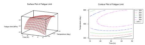
(a) 3D surface plot and contour for fatigue strength with nitriding time and temperature
