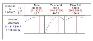
Figure 8: Optimization chart of gas nitriding process for maximum fatigue strength
