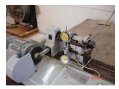
Figure 4: Avery-Denison fatigue testing machine
