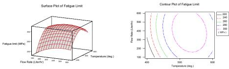
(c) 3D plot and contour for fatigue strength with nitriding temperature and flow rate
