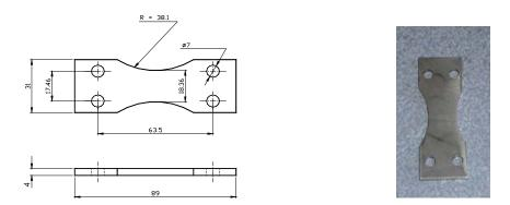
Figure 3: Fatigue test specimen (all dimensions are in millimetres)
