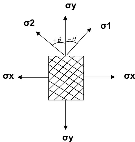
Figure 2: coordinate systems for composite laminate.
