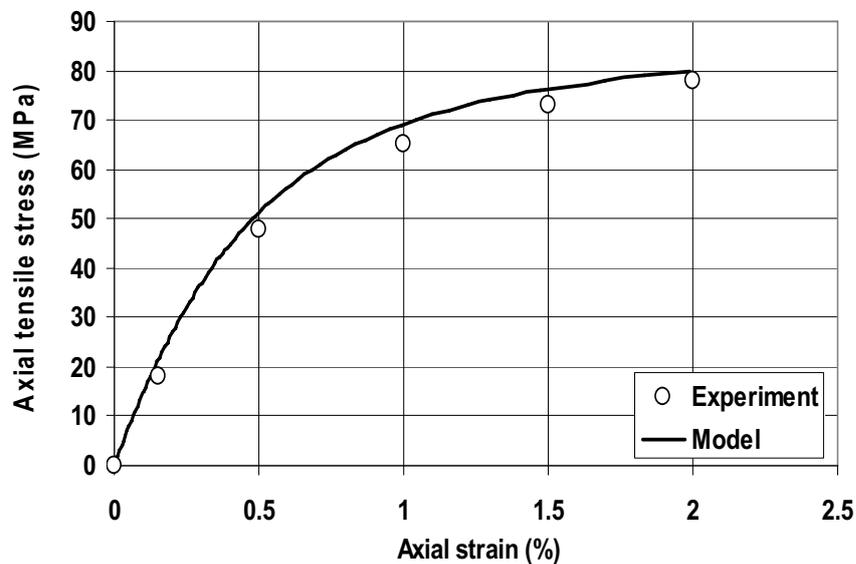
**Figure 7: Modeled and experimental stress-strain curves for  $\pm 45$  angle ply laminate made from glass/ MY750HT917/DY063 under uniaxial tensile loading [19].**
