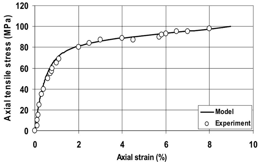
**Figure 6: Modeled and experimental stress-strain curves for  $\pm 45^\circ$  Kevlar/polyester angle ply laminate under uniaxial tensile loading [16].**
