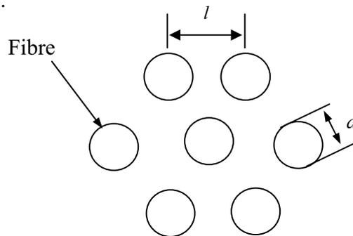
**Figure 3: Hexagonal packing of unidirectional fibres [17].**
