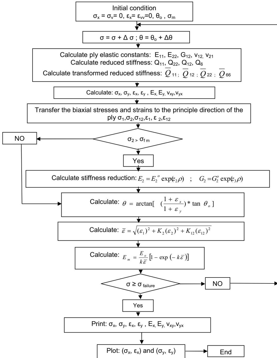
**Figure 4: Flow chart of the model iteration.**
