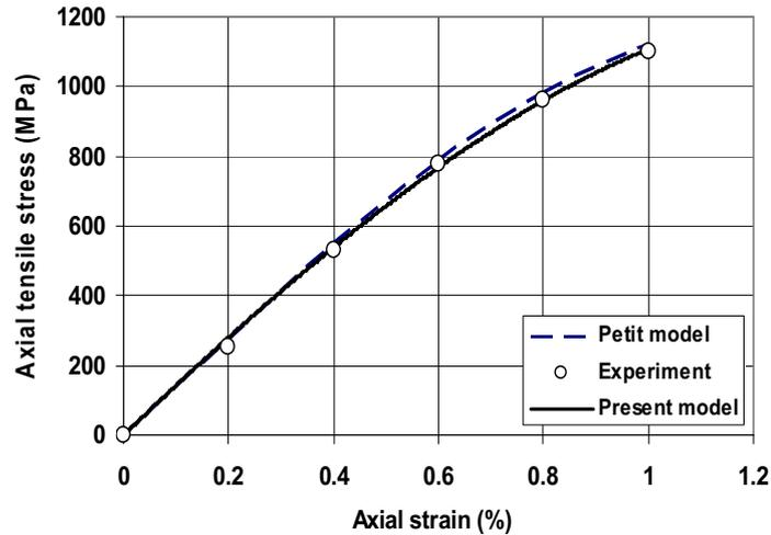
**Figure 10: Modeled and experimental stress-strain curves for  $\pm 20^\circ$  boron/epoxy angle ply laminate under uniaxial tensile loading [2, 21].**
