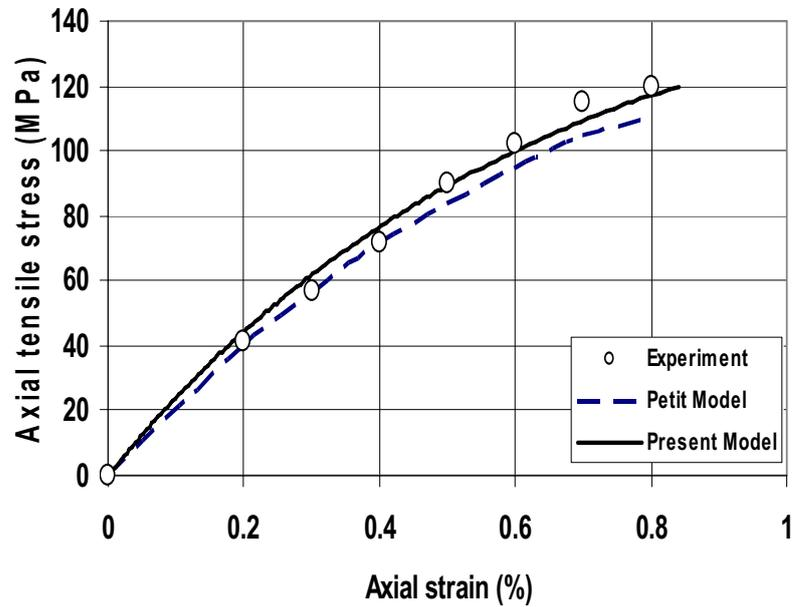
Figure 8: Modeled and experimental stress-strain curves for  $\pm 60^\circ$  boron/epoxy angle ply laminat under uniaxial tensile loading [2, 21].
