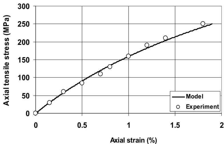
**Figure 11: Modeled and experimental stress-strain curve for  $\pm 55^\circ$  filament wound glass/polyester composite pipe subjected to internal pressure at room temperature [16].**
