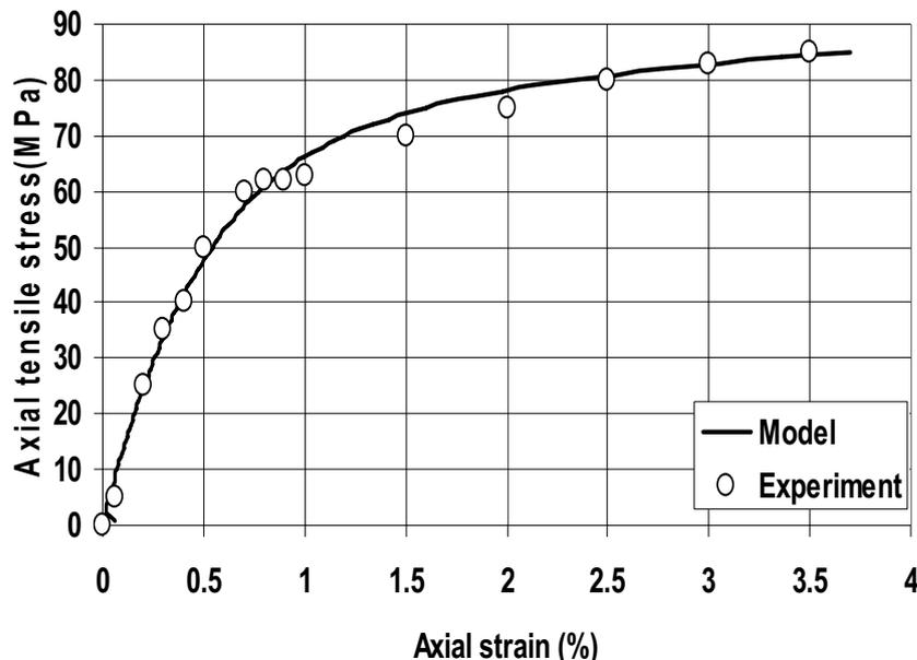
**Figure 5: Modeled and experimental stress-strain curves for  $\pm 45^\circ$  glass/polyester angle ply laminate under tensile loading [16].**
