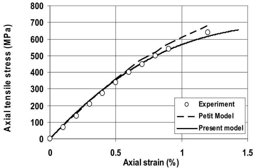
Figure 9: Modeled and experimental stress-strain curves for  $\pm 30^\circ$  boron/epoxy angle ply laminate under uniaxial tensile loading [2, 21].
