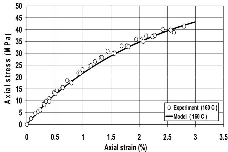
**Figure 12: Modeled and experimental stress-strain curves for  $\pm 55^\circ$  filament wound glass/phenolic (PSX) composite pipe under pure axial loading in wet condition at 160°C [16].**
