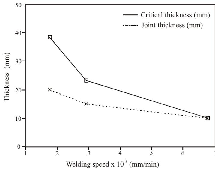
**Figure 4: Comparison of critical thickness with real joint thickness**
