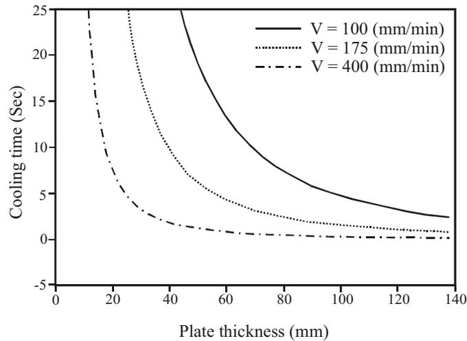
**Figure 3: Shows the effect of welding speed and plate thickness on cooling time**
