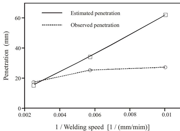
**Figure 7: Comparison of observed and predicted weld depth for various welding speeds.**
