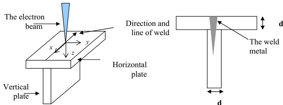
**Figure 1: Shows the joint design, the electron beam, the weld line and the coordinate system**
