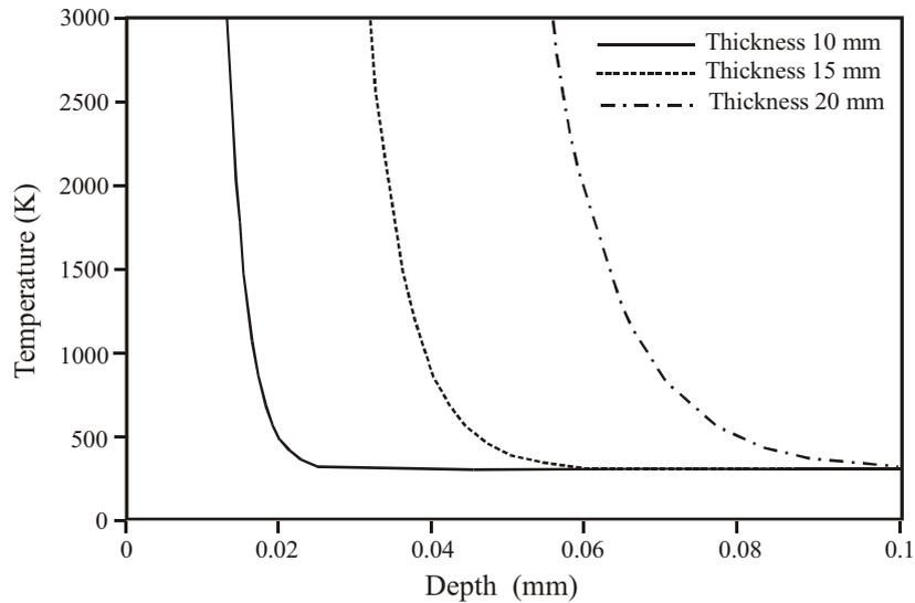
**Figure 5: Peak temperatures versus depth for the three joints**
