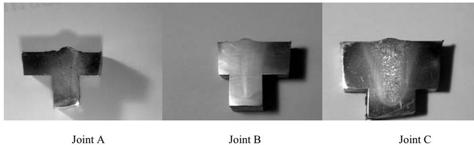
**Figure 6: Macrostructure of cross sections for the three joints**
