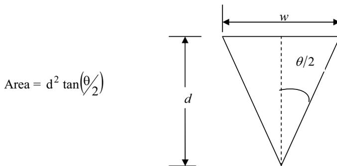
**Figure 8: schematic drawing representing the molten metal in a welded joint.**
