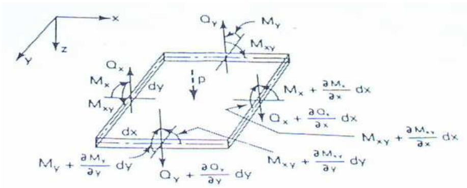
**Figure 2: positive moments, shear forces, and lateral load on plate element**
