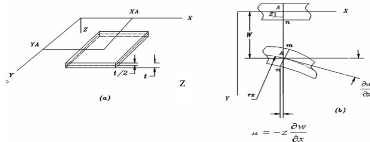
Figure 1: Geometry of undeformed and deformed ( $x, z$ ) plane for classical plate theory
