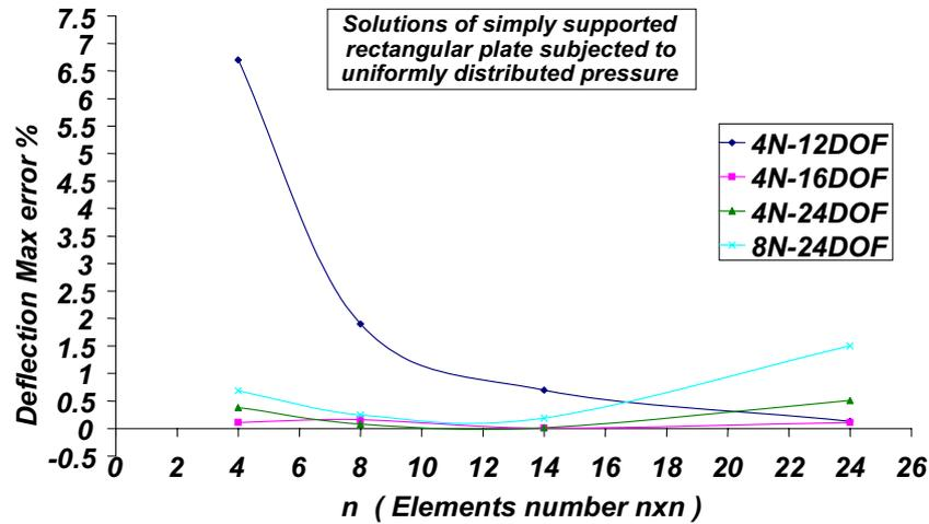
Figure 4: effect of mesh refinement on accuracy [5]
