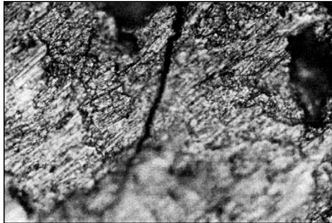
Figure 7: Features of a large disc- Shaped particle x200 showing cracked layered structure with indication of SiC
